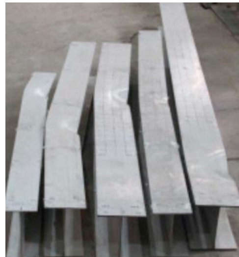
Fig.5 Buckling of 6063 aluminum
